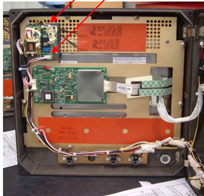
Figure 2.3: Proper routing and cable tying of wires
