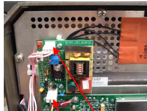
Figure 1.3: Before rotation of inverter
