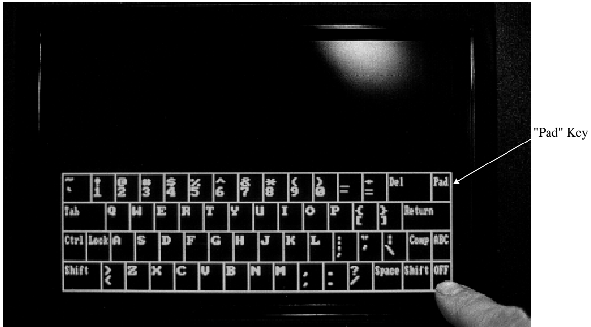
Accessing the QWERTY Keyboard By Touching The Lower Right Corner of the Touch Screen
